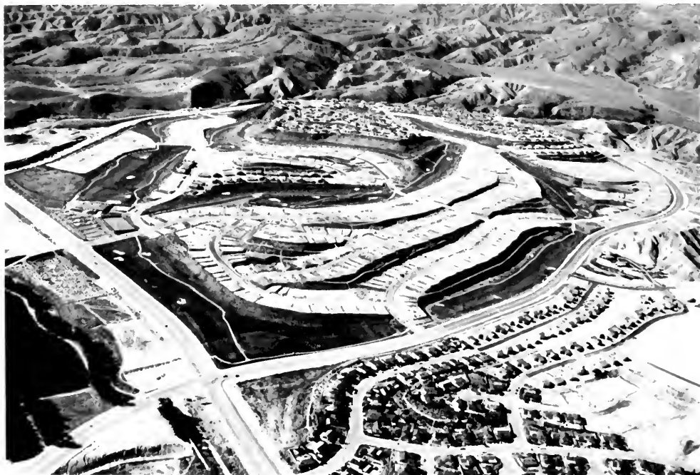
Photo 28. Aerial photograph of Parter Ranch trace of Santa Susana fault zone, which is located at rear of the mesa visible in upper right of photograph. The mesa will be eventually used for building, but the fault zone and area above (upper plate) will be retained as open space. Courtesy of the City of Los Angeles Department of Building and Safety.
